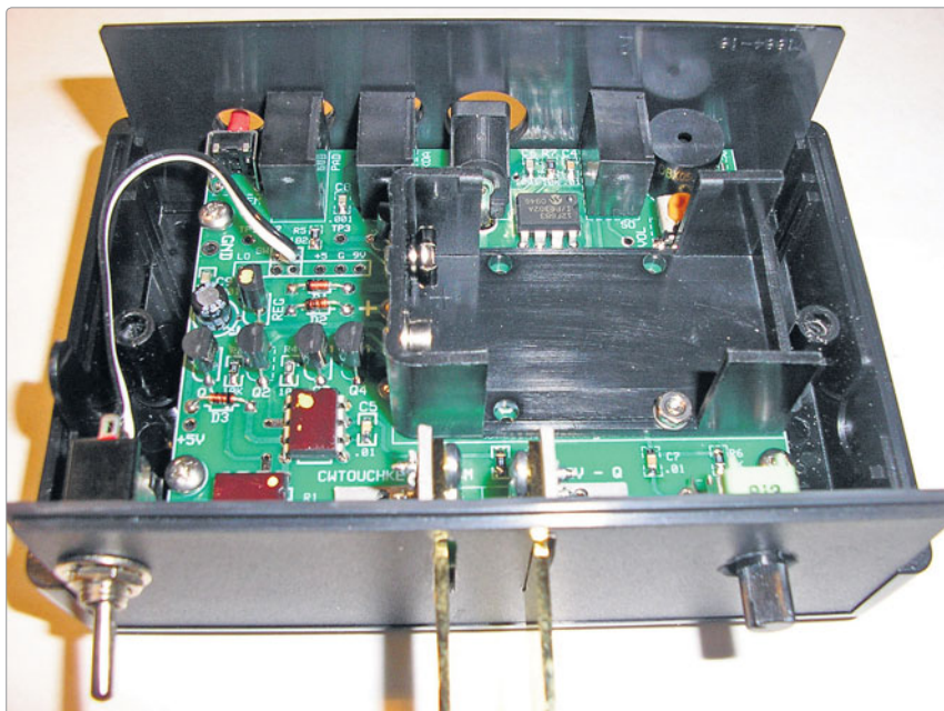
Photo 3: The completed PCB inside its custom enclosure. Note space for the internal 9 V battery, which is optional.
